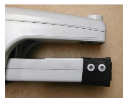
**Step 6 (Optional).**We recommend adding clear tape along the folds of the mask to increase longevity and stability on the MultispeQ.
