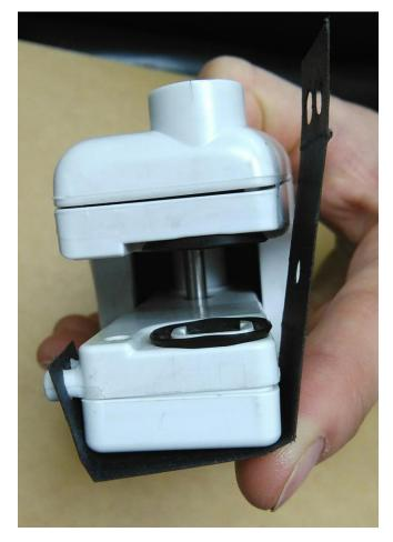
**Step 4.** Continue wrapping the mask around the bottom jaw of the device so it covers the light guide.
