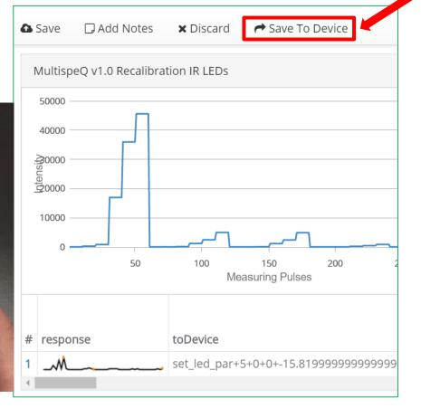
•Step 8. Select *MultispeQ v1.0 SPAD Recalibration (B)* and follow steps 6-7, making sure to enter the value on the front of the SPAD Recalibration Cards envelope. To confirm a quality calibration, check your spad3 r2 value, it should be near 1
