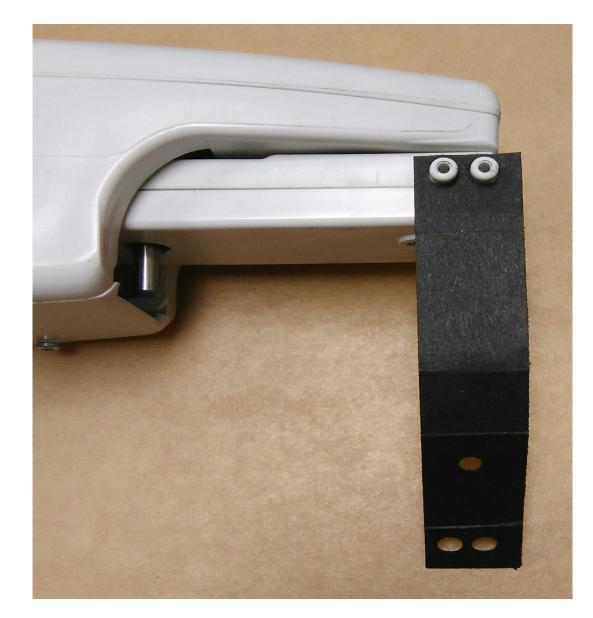
**Step 3.** Fold the mask around the bottom jaw of the device.
